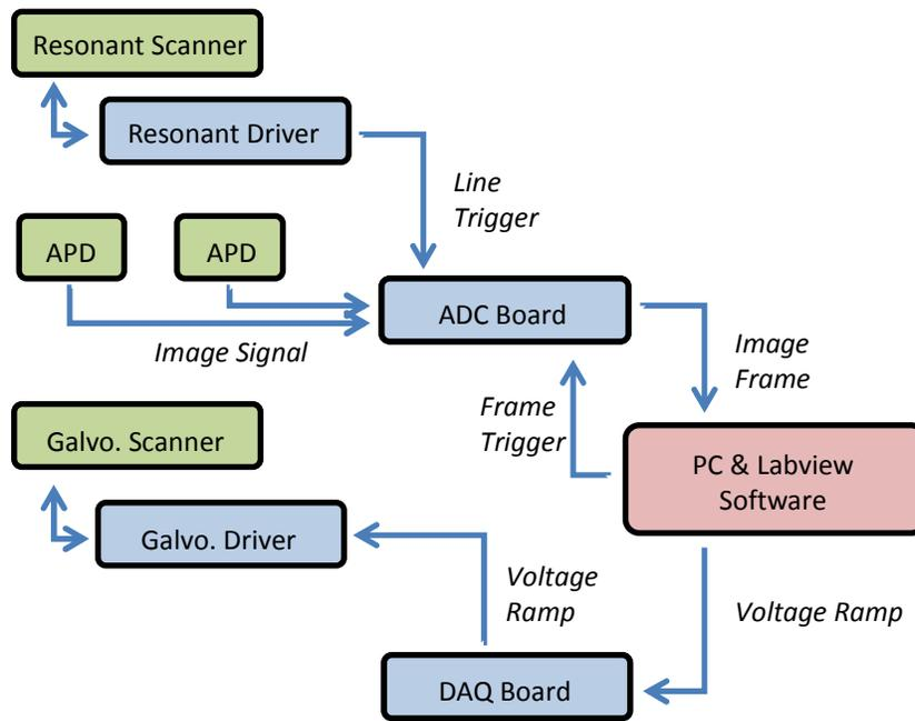
Figure 2. Schematic of galvo control and signal processing scheme. ADC: analogue to digital converter; APD: avalanche photodiode.
