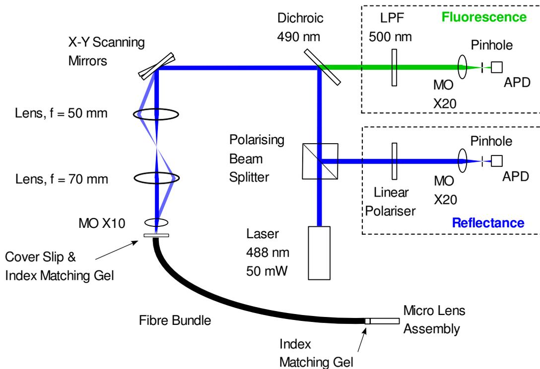
Figure 1. Optical layout for dual mode endomicroscopy system. MO: microscope objective; LPF: long pass emission filter; APD: avalanche photodiode.
