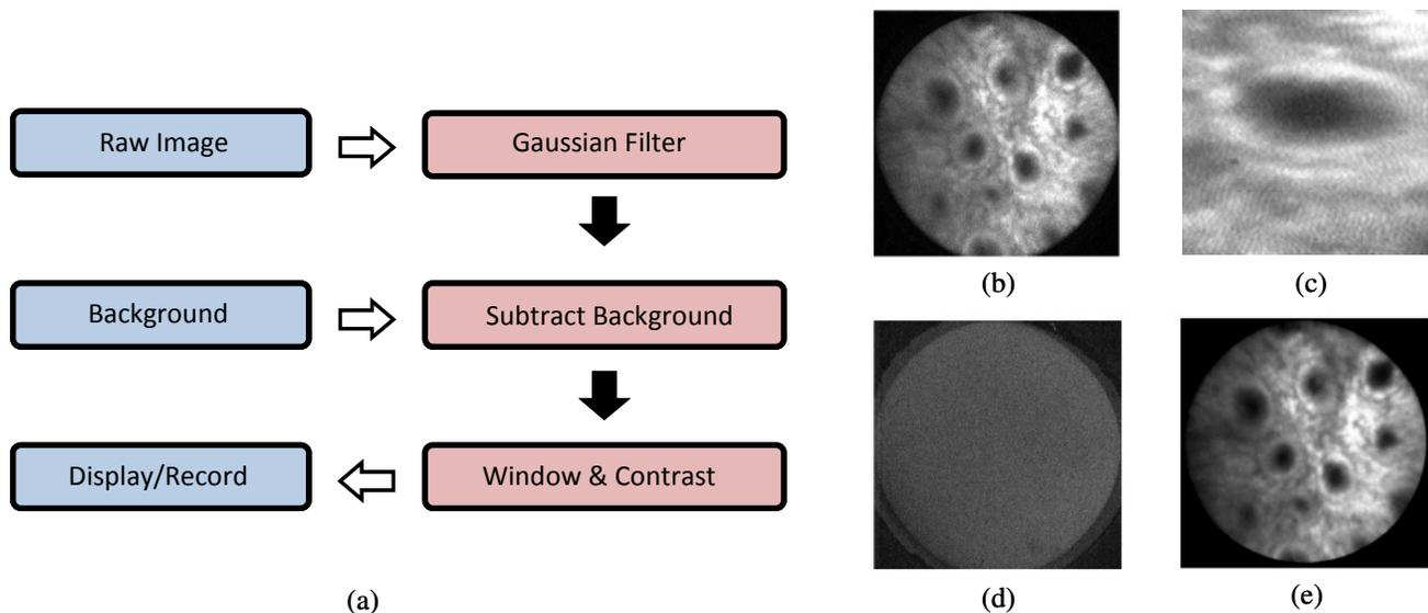
Figure 3. Illustration of real-time image processing scheme. (a) Flow diagram showing processing steps; (b) example raw image (porcine small bowel, fluorescence channel); (c) zoom in on raw image showing honeycomb pattern; (d) background image showing autofluorescence; (e) processed image.
