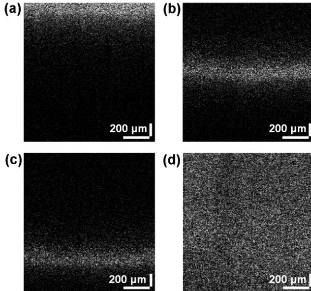
**Fig. 2:** B-scan of diluted milk shown without dynamic focus with focus at (a) top of scan (b) centre of scan, (c) bottom of scan, and (d) with dynamic focus.
