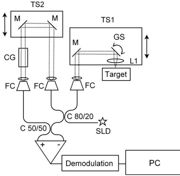
**Fig. 1:** TD-OCT with dynamic focus. L1: lens ( $f = 15$  mm), M: mirror, FC: fibre collimator, C: 2x2 coupler, GS: XY galvo scanner head, CG: dispersion compensating glass; SLD: superluminescent diode; TS1: translation stage for depth scanning with dynamic focus; TS2: translation stage for depth scanning (no dynamic focus).
