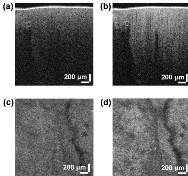
**Fig. 3:** Scans of tooth enamel layers; (a) B-scan without dynamic focus, (b) B-scan with dynamic focus, (c) C-Scan (en-face) without dynamic focus, (d) C-scan with dynamic focus.
